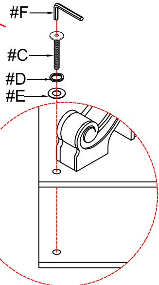
Adjust leveler according to ground level.
