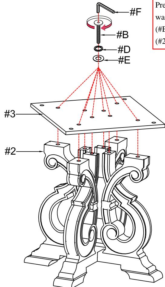
Prepare 8 bolts assembly by inserting lock washer (#D), then flat washer (#E) onto bolts (#B). Align shelf (#3) to the holes of the legs (#2), then secure by using bolts (#B).
