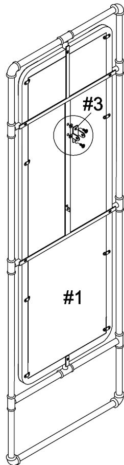
Align support plate (#3) to the holes of the mirror (#1), then secure by using bolts (#A) with washers (#E).
