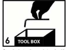
Save the instructions and store the Allen wrench or any supplied tool for later maintenance. After two weeks, check and tighten any loose hardware and repeat again every six months thereafter.
