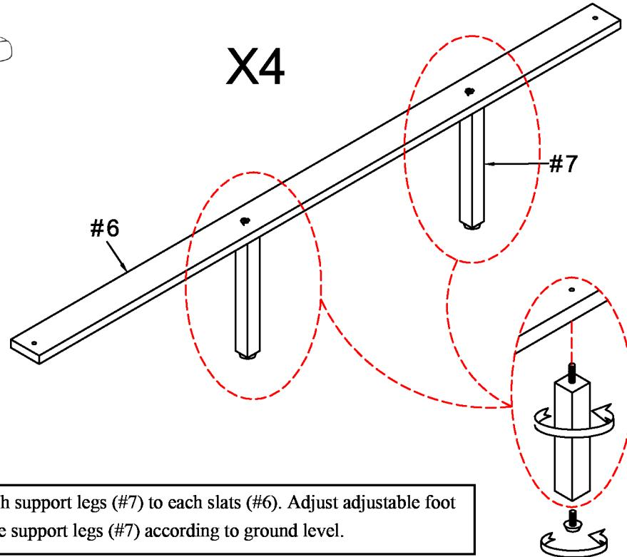
Attach support legs (#7) to each slats (#6). Adjust adjustable foot on the support legs (#7) according to ground level.
