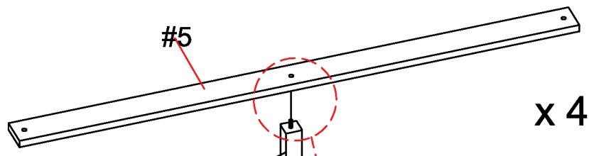
Insert the threaded ends of the bed slat supports (#6) into the holes along the bed slats (#5). Turn right to tighten.
