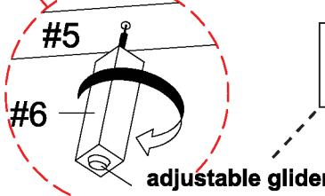
Adjust according to ground level.
