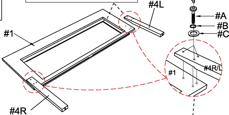
2. Prepare 6 bolt assemblies by inserting a lock washer (#B) onto the bolt (#A) then a flat washer (#C) onto that same bolt (#A). Insert 3 into each leg and secure using the Allen wrench.
