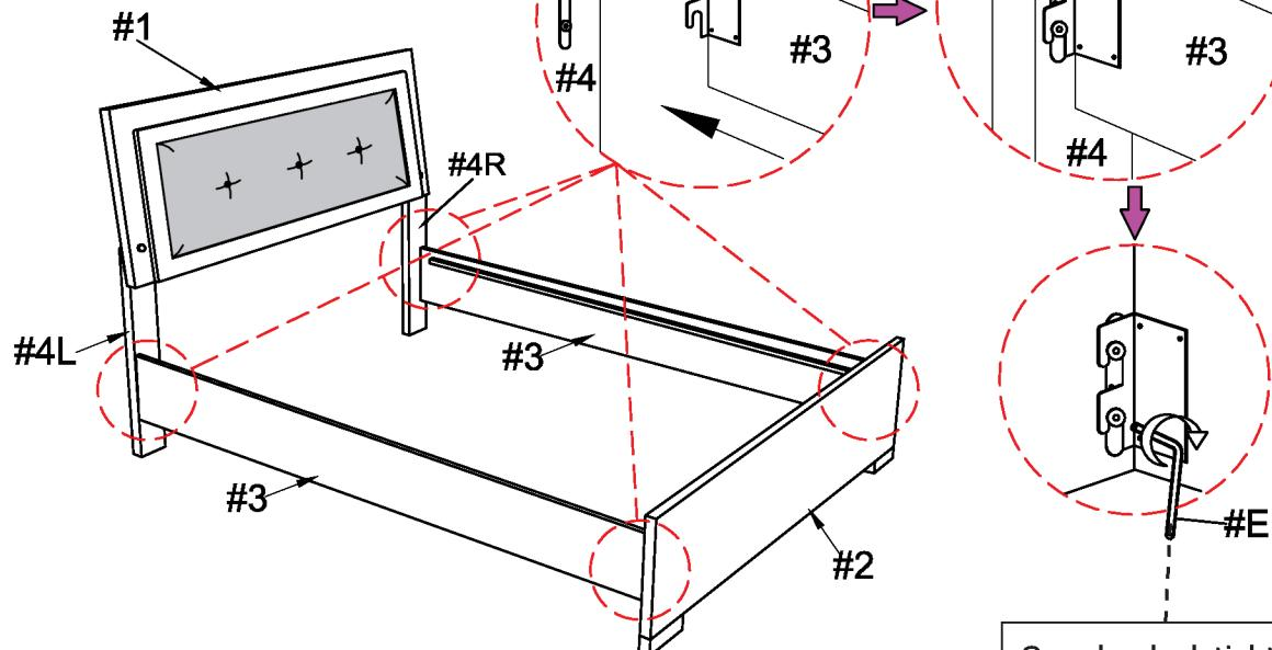
Once hooked, tighten bolts using the Allen wrench (#E).
