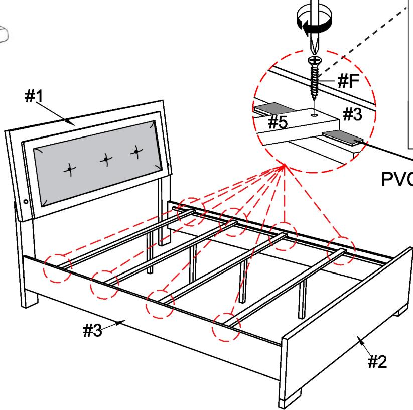
Place each end of the slats (#5) onto a Pvc stopper , then place onto the side rails (#3). Insert a screw (#F) into each end. Secure using a Phillips screwdriver.
