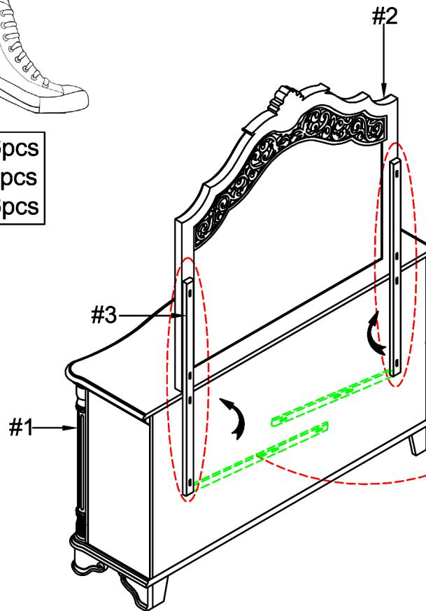
Prepare 6 bolts assembly by inserting lock washer (#B), then flat washer (#C) onto bolts (#A). Align mirror support (#3) to the holes of the mirror (#2) and dresser (#1). Secure by using bolts (#A).
