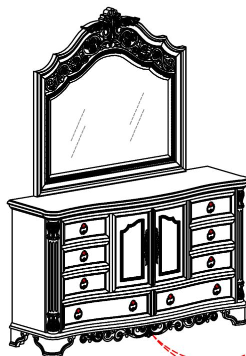
Attach support leg (#4) to the bottom middle hole of the dresser. Adjust leveler of the support leg (#4) according to ground level.
