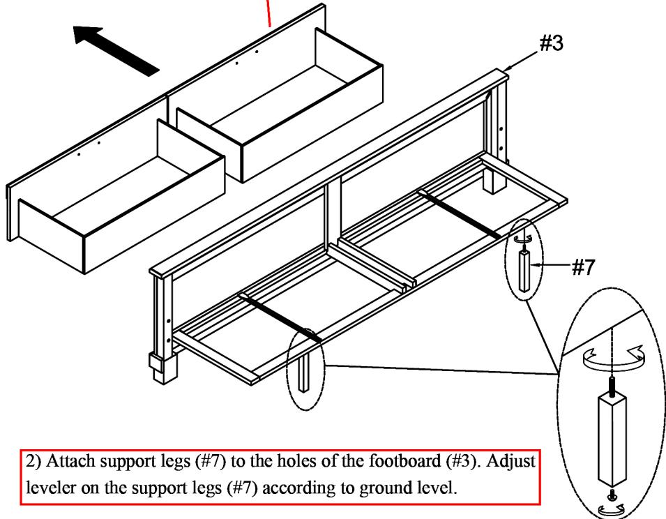
2) Attach support legs (#7) to the holes of the footboard (#3). Adjust leveler on the support legs (#7) according to ground level.
