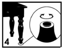
Some furniture comes with height adjusetment knobs underneath each leg. To lower or to raise each leg, you need to turn clockwise or counterclockwise, respectively.
