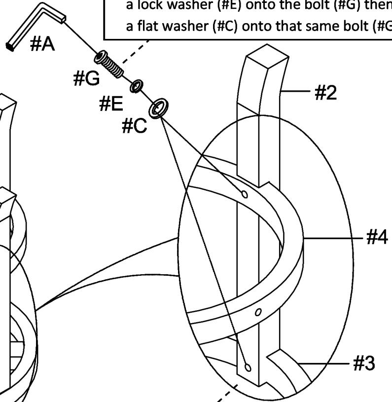
2. Align the fourth leg (#2) to the holes along the sides, then insert the bolts from within and secure using the Allen wrench (#A).
