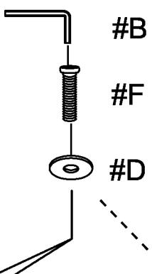
3. Prepare 4 bolt assemblies by inserting a flat washer (#D) onto the bolts (#F), then insert those bolts into the holes and secure using the Allen wrench.
