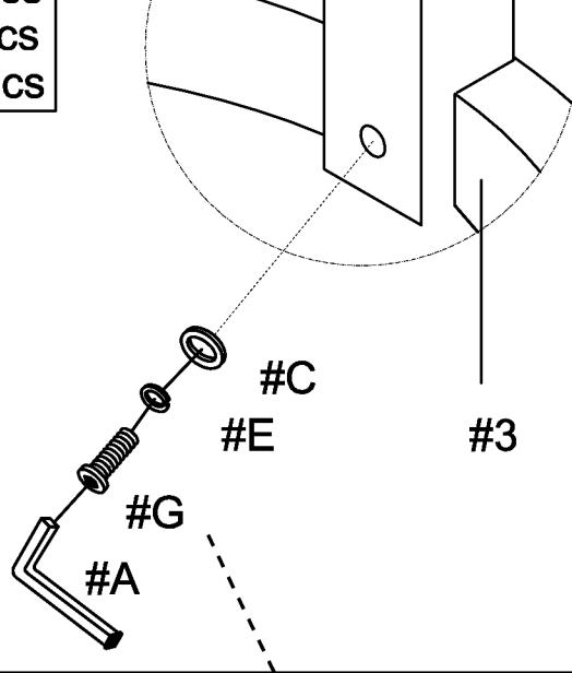
2. Align three legs (#2) to the holes along the seat turnplate (#3), then insert the bolts from within and secure using the Allen wrench (#A).
