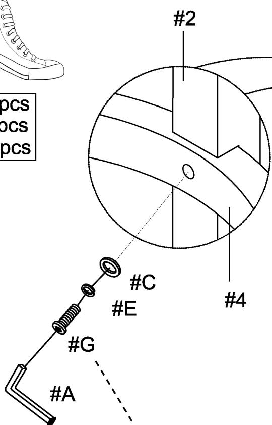
2. Align the leg support (#4) to the holes along the legs (#2), then insert the bolts from within and secure using the Allen wrench (#A).
