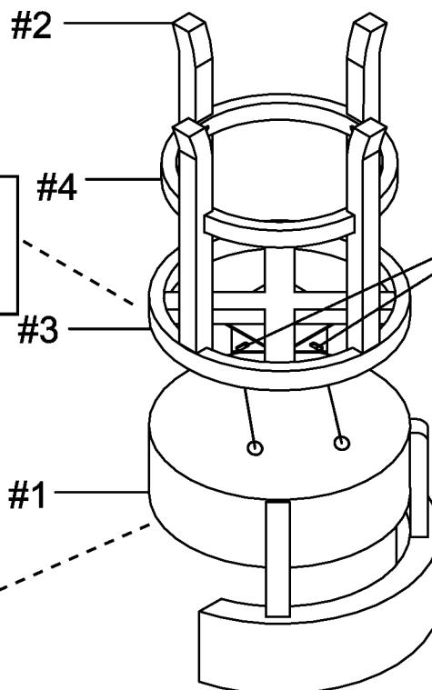
2. Align the seat turnplate (#3) face down to the holes along the bottom of the seat (#1).
