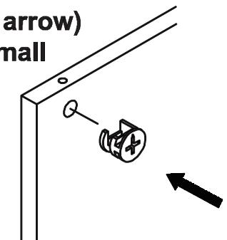
Insert the cam lock bolt into the pre-drilled hole above the cam connector.
