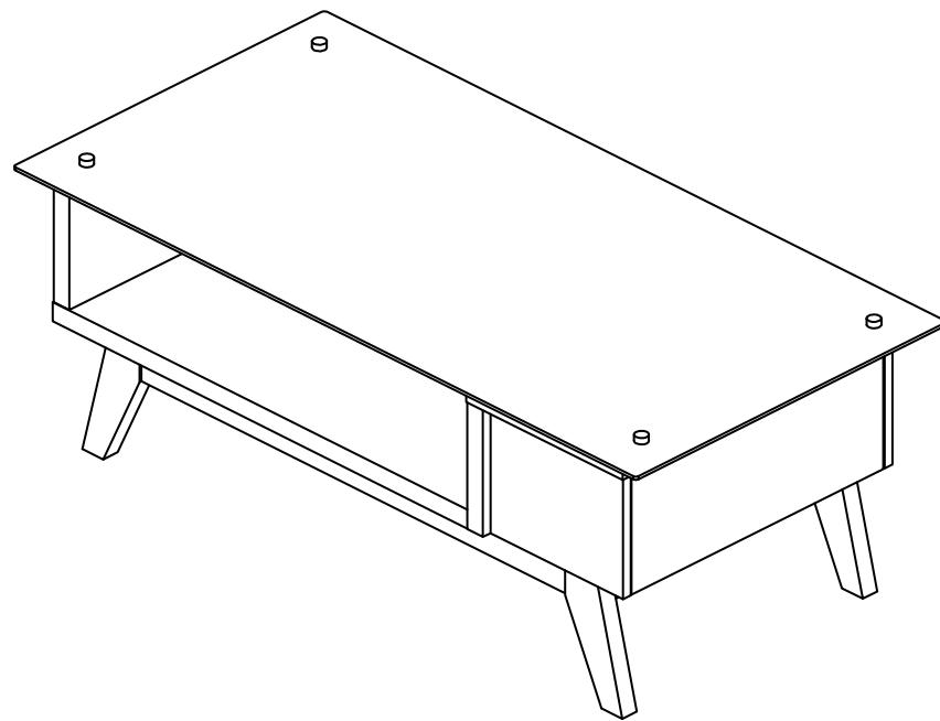
Make sure the unit is rested on a flat surface and does not feel loose or wobbly. If it does, double check all bolts/screws are secured and properly tightened.
