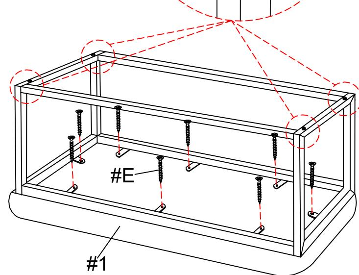
1) Align the seat cushion (#1) to the holes of the top metal rails (#4) and side metal frames (#2). Secure with screws (#E). There will be no pre-drilled holes on the seat cushion (#1).
