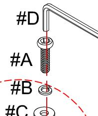
Prepare 16 bolts assembly by inserting lock washer (#B), then flat washer (#C) onto bolts (#A). Secure all the holes with bolts (#A).
