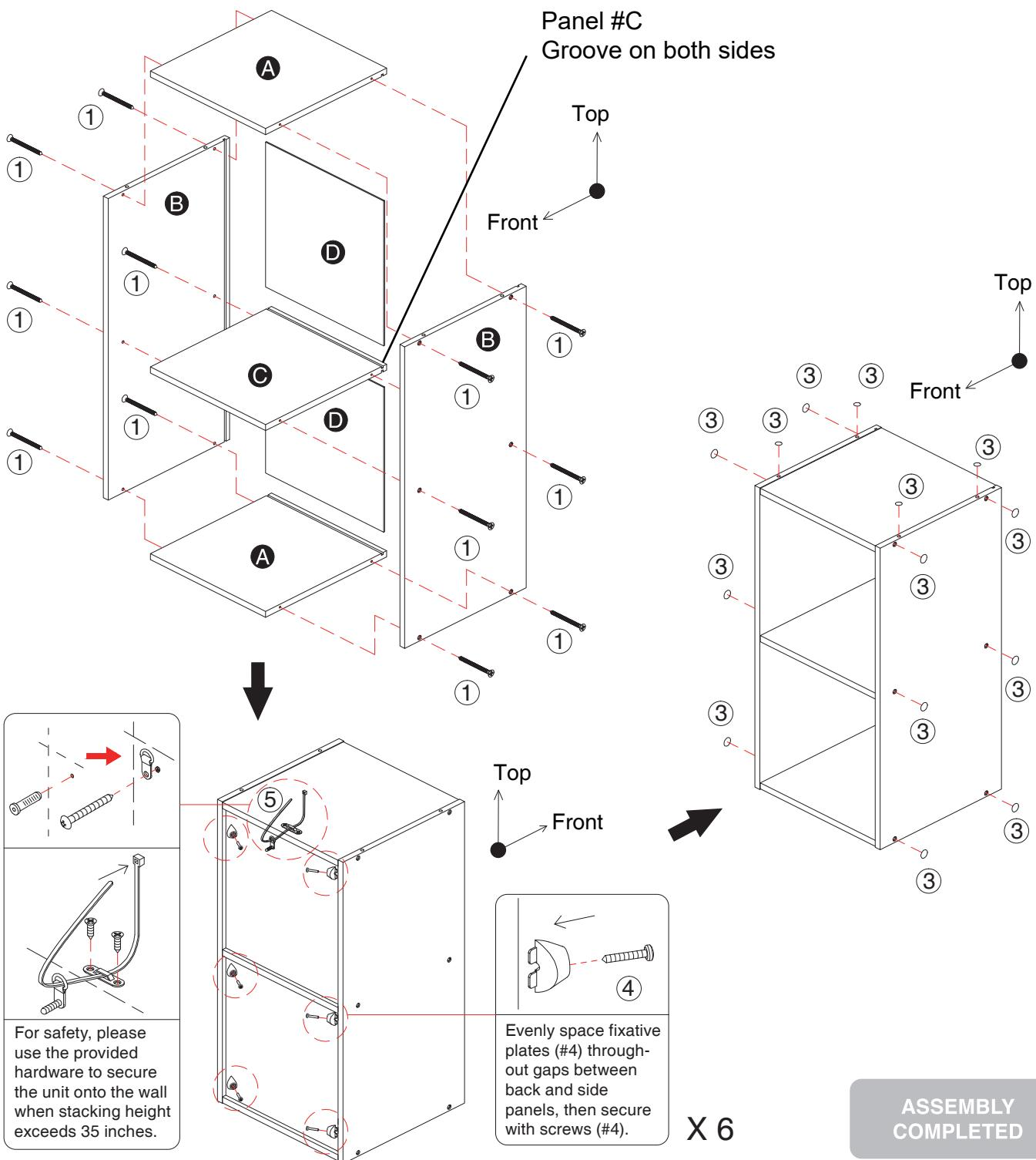
For safety, please use the provided hardware to secure the unit onto the wall when stacking height exceeds 35 inches.
