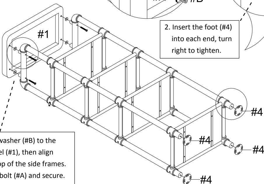
1. Align a washer (#B) to the top panel (#1), then align to the top of the side frames. Insert a bolt (#A) and secure.
