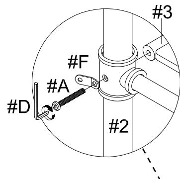
Align the shelves (#3) to the holes along the side frames (#2), then insert a bolt (#A) into each hole. Secure using the Allen wrench.
